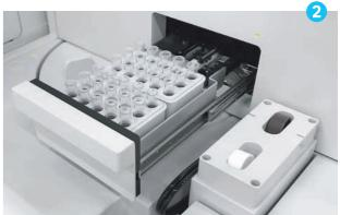
Easily replenish the dedicated measurement cuvettes used in the CLEIA\* unit by installing the entire tray.
